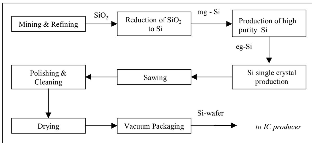
**Figure 1.** A simplified flow chart of Si-wafer production.
