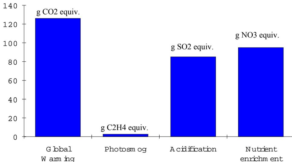
Fig. 1. Environmental effect types for 1 ton of exploited talc (mining + transport to the plant)
